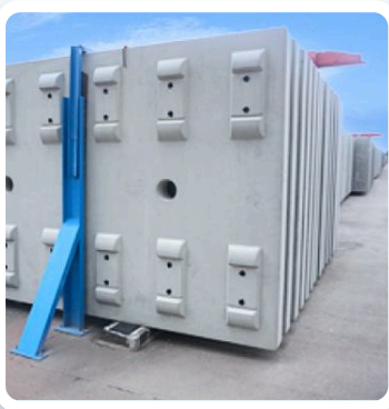
Railway Track Slab
